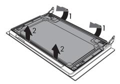
4. Lift the intermediate glass unit upwards.
