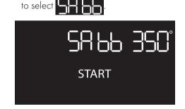
6. Turn the temperature knob to the right or left to select the required temperature.
