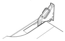
Grasp the door on both sides with both hands, lift it forming an angle of around 30° and remove it.
