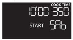
2. Turn the temperature knob to the right or left to set the required cooking time (from 10 minutes to 73 hours).
