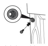
4. Cover the bushings with the covers removed previously.
