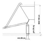
It is important to prevent the hose from coming loose and falling. For this purpose, the plastic support is equipped with a hole for tying it to the wall or water tap. The free end should be positioned at a height of between **30 and 100 cm (11" 13/16 and 3' 3" 3/8)**, and should never be submerged in water. If a horizontal drain extension hose is used (for a maximum 3 m - 9' 10" 7/64 ), the drain hose can be placed at a maximum height of.**85 cm** (2' 9" 15/32) from the ground.
