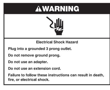
Before you move your refrigerator into its final location, it is important to make sure you have the proper electrical connection.
