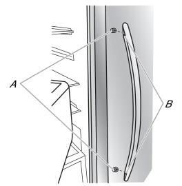
A. Shoulder screws B. Setscrews inside the handle
