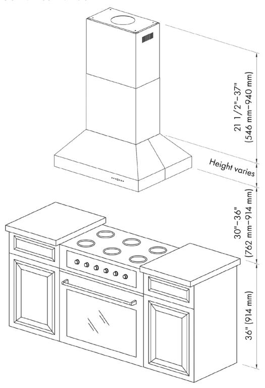
NOTE: The recommended height to install your hood is 30" (762 mm) minimum and 36" (914 mm) maximum above your range top or cook top. For outdoor installation, the hood should be installed between 36" (914 mm) and 42" (1067 mm) above the grill. These distances allow for optimal venting efficiency. The height of your chimney will vary depending on model of hood, as well as the height of your kitchen ceiling. Consult an HVAC or installation professional for ventilation advice.
