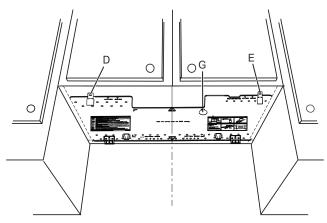
**NOTE:** If upper cabinet is metal, the supply cord bushing needs to be installed around the supply cord hole as shown.
