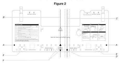
NOTE: If wall studs is within 6" (15.2 cm) of the vertical centerline (see "Mark Rear Wall" section), only recirculation or roof venting installation can be done.
