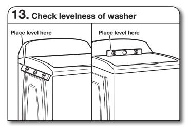
Move the washer to its final location. Place a level on top edges of washer. Use side seam as a guide to check levelness of sides. Check levelness of front using lid, as shown. Rock washer back and forth to make sure all four feet make solid contact with floor. If washer is level, skip to step 15.
