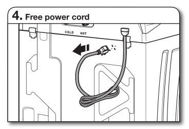
Firmly grasp power cord plug and pull to free from rear panel. Gently place power cord over console to allow free access to back of washer.
