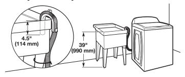
Minimum capacity: 20 gal. (76 L). Top of laundry tub must be at least 39" (990 mm) above floor; install no higher than 96" (2.44 m) from bottom of washer.
