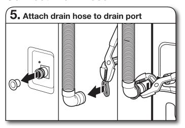
Remove the red plastic plug from the black drain port on the back of the washer.
