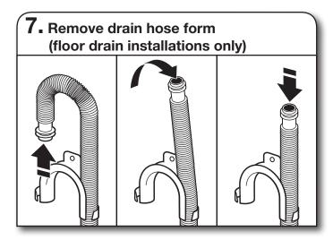
For floor drain installations, you will need to remove the drain hose form from the end of the drain hose. You may need additional parts with separate directions. See the "Tools and Parts" section.
