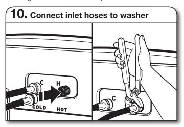
Attach hot water hose to hot water inlet valve marked with a red ring. Screw coupling by hand until it is snug. Use pliers to tighten couplings an additional two-thirds turn. Repeat with cold water inlet valve.
