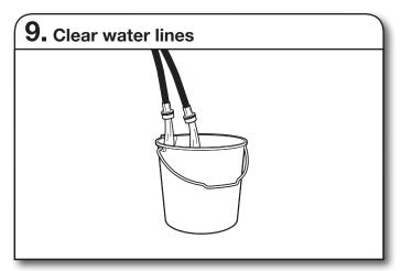
Run water for a few seconds through hoses into a laundry tub, drainpipe, or bucket to avoid clogs. Water should run until clear. Make note of which hose is connected to hot water to help in attaching hoses to washer correctly.
