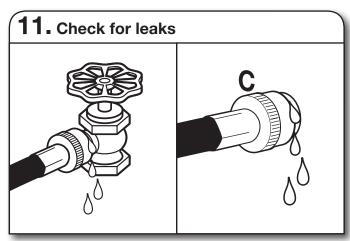
Turn on water faucets to check for leaks. A small amount of water may enter washer. It will drain later.
