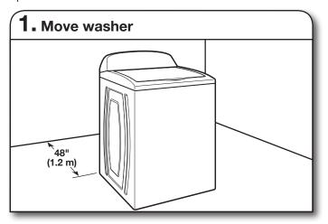
Move washer to within 4 ft. (1.2 m) of its final location; it must be in a fully upright position.
