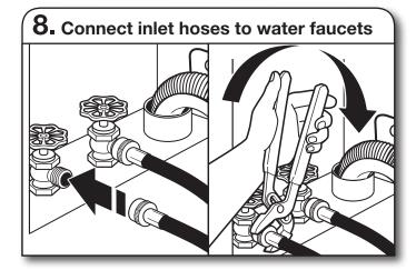
Attach hose to hot water faucet. Screw on coupling by hand until it is seated on washer. Use pliers to tighten couplings an additional two-thirds turn. Repeat this step with second hose for cold water faucet.
