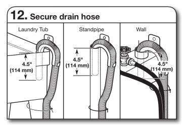
Secure drain hose to laundry tub leg, drain standpipe, or inlet hoses for wall standpipe with cable tie.
