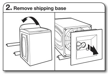
To avoid damaging floor, place cardboard supports from shipping carton on floor behind washer. Tip washer back and place on cardboard supports. Remove shipping base. Set washer upright.
