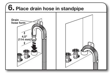
Place hose into standpipe (shown in picture) or over side of laundry tub.
