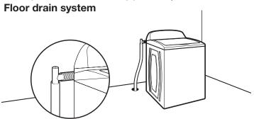
Floor drain system requires a Siphon Break Kit (Part Number 285834), 2 Connector Kits (Part Number 285835), and an Extension Drain Hose (Part Number 285863) that may be purchased separately. To order, please see toll-free phone numbers in "Assistance or Service" section. Minimum siphon break: 28" (710 mm) from bottom of washer. (Additional hoses may be needed.)
