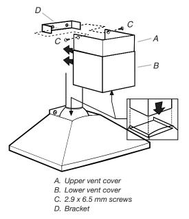
NOTE: For vented installations, the upper vent cover may be reversed to hide slots.
