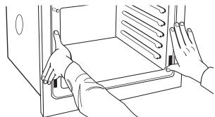
Push oven completely into cabinet and center oven into cabinet cutout.  Securely fasten the oven to the cabinet using the #8-14 x 3/4" screws provided.
