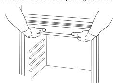
Push against the seal area of the front frame to push the oven into the cabinet until the back surface of the front frame touches the front wall of the cabinet.
