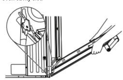
IMPORTANT: Do not close the door at this step or damage may occur to the door hinge.
