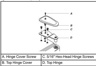
Adjust the door so that the bottom of the refrigerator door is aligned with the top of the freezer drawer. Tighten all screws.
