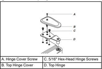
2. Replace the parts for the bottom hinges as shown below. Tighten screws. Replace the refrigerator doors.
