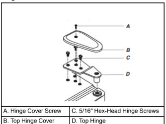
**4.** Remove the center hinge pin and remove the hinge screws as shown below. Lift the freezer door free from the cabinet.
