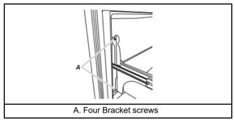
3. Lift drawer front upward and off the screws.
