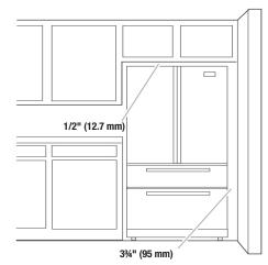
To ensure proper ventilation for your refrigerator, it is recommended to allow a 1/2" (1.27 cm) space on each side and at the refrigerator top. Allow at least 1" (2.54 cm) between back of cabinet and the wall (consider the condenser as back in case is present). If your refrigerator has an ice maker, make sure you leave extra space at the back for the water line connections.
