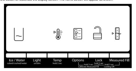
For your convenience, your refrigerator and freezer controls are preset at the factory. When you first install your refrigerator, make sure that the controls are still set to the recommended set points. The factory recommended set points are 37°F (3°C) for the refrigerator and 0°F (-18°C) for the freezer.
