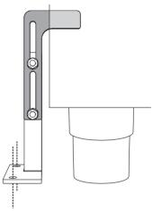
4. Lower the bracket attachment until anchoring the appliance slot, tighten the nuts previously assembled. The anti-tip device works properly only if the bracket attachment is securely anchored to the appliance.
