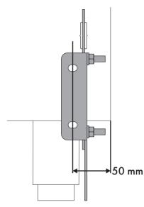
Move the bracket onto the wall and mark the position of the holes to be drilled in the wall.
