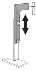
3. After having positioned and leveled the appliance, move the bracket close to the rear of the appliance and anchor it to the floor.
