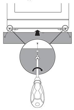
3. Fasten the front skirting to the appliance using the previously removed screws.
