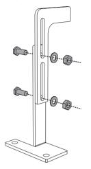
2. The bracket attachment should insert into one of the central slots at the rear.
