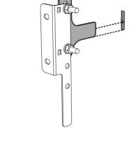
3. Align the base of the fastening bracket with the ground and tighten the screws to fix the measurements.
