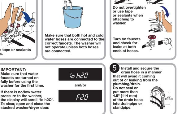
Make sure that the washer/dryer is level (see the "Leveling Stacked Washer/Dryer" section in the Installation Instructions). Run a wash cycle to verify that the washer is working correctly and has no leaks at faucets and inlet hoses.
