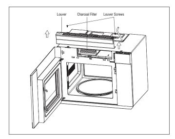
**3.** Slide louver to the left and pull it straight out.
