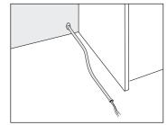
Remove 2" - 3" (51mm-76mm) of house line wire from its outer casing and then remove 3/8"-1/2" (10mm - 13mm) of insulation from each wire.
