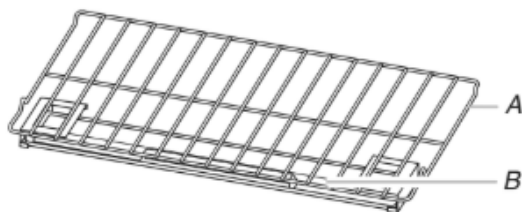
A. Steam rack B. Water reservoir
