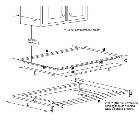
Overhead cabinet should not exceed a maximum depth of 13" (330 mm).
