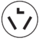
3-wire receptacle (10-30R)
