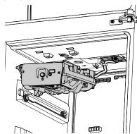
6. Reinstall the cover over the connector and the ice maker wire by inserting the back of the cover as indicated. Then rotate the cover upward and snap it into the housing. After the cover is snapped into the housing, insert screw to secure the cover.
