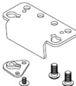
Figure 7a - Lower Hinge Bracket (Before Reversal)
