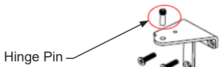
Figure 6 - Upper Right Hinge Orientation (Before Reversal)
