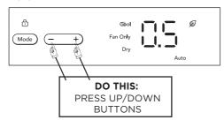
Note: For Delay Stop or Start, press the Timer button when the unit is in the On or Off position. Then tap or hold the " – " or " + " button to change delay timer at 0.5 hour increments, up to 10 hours, then at 1 hour increments up to 24 hours. After 5 seconds, the control will count down the time remaining until Stop or Start (8h, 7.5h, 7h, etc.).
