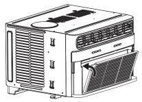
3. Reinstall the Dust filter and air inlet grille.
