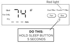
After 1440 hours of operation the PureAir<sup>™</sup> Filter indicator will turn red. To reset, replace with new PureAir<sup>™</sup> Filter, then hold the "Sleep" button 5 for seconds.
