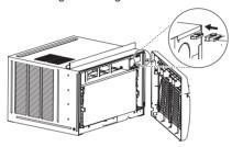
Attach the front grille to the cabinet by inserting the tabs on the grille into the slots on the front top of the cabinet. Push the grille in until it snaps into place.
