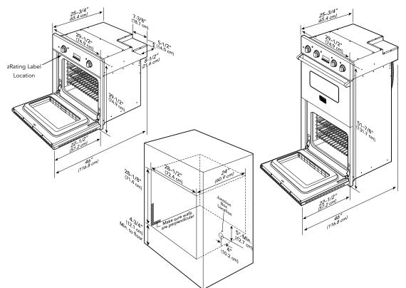
Note: A minimum of 2" (5.1 cm) spacing above and below the oven to any adjacent appliances such as a microwave or warming drawer is required for ventilation purposes.
