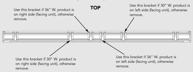
**\*NOTE:** Depending on unit configuration, two brackets should be removed and discarded. The 72" W. and 60" W. grille assemblies have all four (4) brackets mounted in the proper location.
