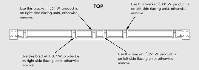
**\*NOTE:** Depending on unit configuration, two brackets should be removed and discarded. The 72" W. and 60" W. grille assemblies have all four (4) brackets mounted in the proper location.
