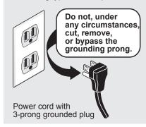
CIRCUIT - Individual, properly polarized and grounded 15 amp. branch circuit fused with 15 amp. time delay fuse or circuit breaker.
