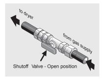
Check for gas system leaks with a manometer. If a manometer is not available, test all connections by brushing on a soapy water solution.
