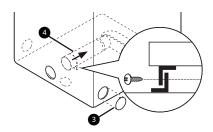
Preassemble a 4" (10.2 cm) elbow **5** to the next 4" (10.2 cm) duct section, and secure all joints with duct tape. Be sure that the male end of the elbow faces AWAY from the dryer. Insert the elbow/duct assembly through the side opening and press it onto the adapter duct. Secure it in place with duct tape. Be sure that the male end of the duct protrudes 1.5" (3.8 cm) to connect the remaining ductwork. Attach the cover plate **6** to the back of the dryer with the included screw.
