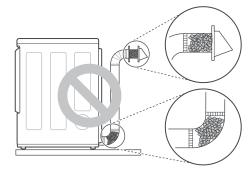
Make sure the ductwork is not crushed or restricted.
