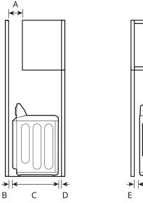
For cabinet installation with a door, minimum ventilation openings in the top of the cabinet are required.
