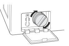
**8** Close the drain pump filter cover.
