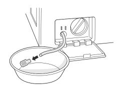
**4** Remove the pump filter.
