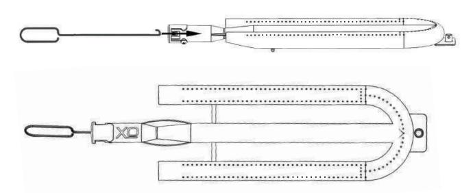
**IMPORTANT:** When replacing the burners care must be taken to ensure the burner venturi is re-centered over the orifice. Failure to do so will result in poor burner performance and will cause ignition problems. If you are unsure how to perform this critical maintenance - call for service.
