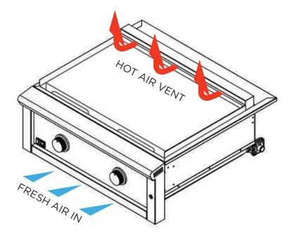
Because the burners are covered by the griddle plate the design of the appliance makes it less susceptable to wind patterns than a grill, however care should be taken to avoid conflicts with strong prevailing wind patterns.
