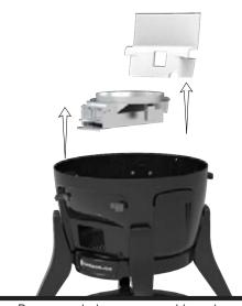
Remove ash drawer assembly and rear insulation. Note - the rear insulation is secured with the ash drawer assembly.
