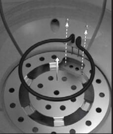
Remove the 2 acorn nuts from the element mounting plate. Then, with extreme caution, lift the element straight up and out of the grill. (NOTE - you may need to lightly hold down the element bracket to remove the element from the bracket).
