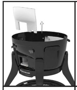
Remove the front insulation.
