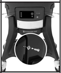
Remove two screws from front module.
