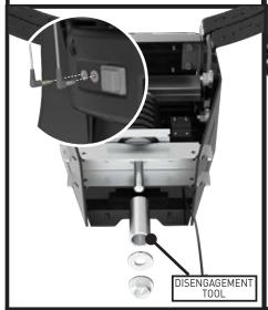
Install the disengagement tool on the hinge. Unplug pit probe, lid switch, and power supply from rear of grill.
