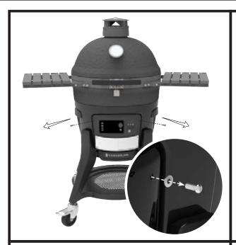
Remove two screws from front module.
