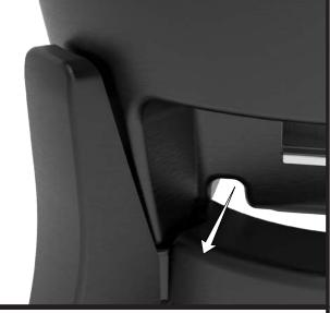
Fish the new wire harness through the rear pass through hole.
