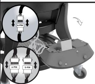
Disconnect the wire harness from the rear module. Use caution do not apply tension on the wire harness. (Note - leave the element wires connected).
