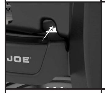
Fish the new wire harness through the front pass through hole.
