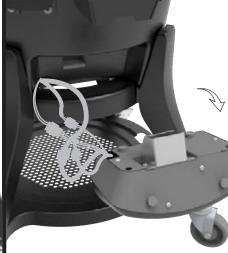
Disconnect the wire harness from the rear module. Use caution do not apply tension on the wire harness. Set the rear module aside, you will need to install this on the new black base kit.
