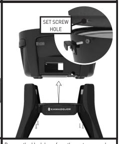
Remove the black base from the cart – remember to remove the 4 screws that connect the grill base to the cart. Note – when installing the ceramic base, line up the hole in the ceramic with the front set screw location on the grill.
