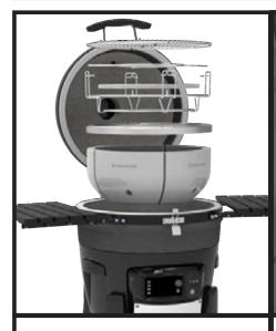
Remove all internal components of the grill. Cooking grates, x rack, heat deflectors, SS ring, ceramic firebowl panels, charcoal grate, element.
