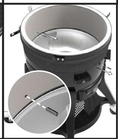
Remove the set screw from the inside of the grill (front).
