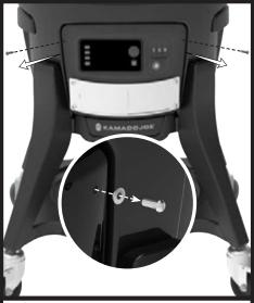
Remove two screws from front module.
