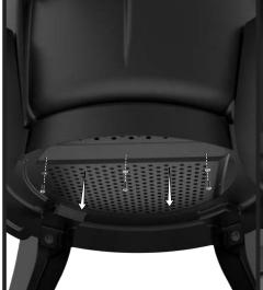
Remove the three wire harness cover screws.
