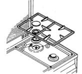
In the event of a momentary power failure, the hob burner can be ignited manually using an igniter.
