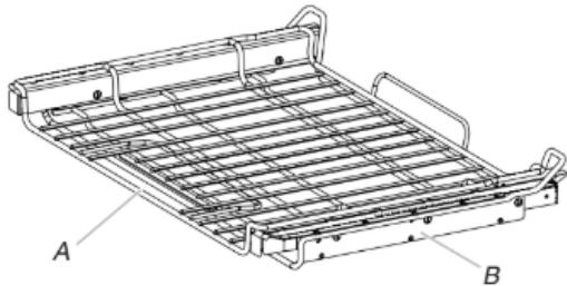
A. SatinGlide™ roll-out extension rack for Smart Oven+ Attachments B. Sliding shelf
