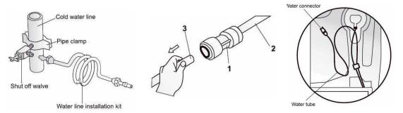
**CONNECT WATER VALVE:** Connect water supply line to water valve with accessible shutoff valve. Connect water line to refrigerator using installation kit. Kit includes one water tube and connector. Second water tube not supplied. Connect first water tube [2] into corresponding hole of water connector[1].
