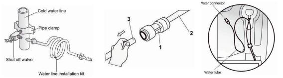
**CONNECT WATER VALVE:** Connect water supply line to water valve with accessible shutoff valve. Connect water line to refrigerator using installation kit. Kit includes one water tube and connector. Second water tube not supplied. Connect first water tube [2] into corresponding hole of water connector[1].
