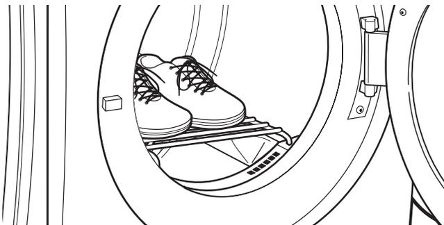
3. Place wet items on top of the drying rack. Allow space around items for air to circulate. The drying rack does not move, but the drum will rotate; be sure to leave adequate clearance between items and the inside of the dryer drum. Make sure items do not hang over the edges or between drying rack grille.
