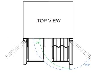
WHEN INSTALLING WITH THE HINGE SIDE NEXT TO A WALL, LEAVE ENOUGH CLEARANCE GAP FOR CABINET HANDLES. DOOR MUST BE ABLE TO OPEN A MINIMUM OF 90° FOR THE SHELVES AND RACKS TO EXTEND.
