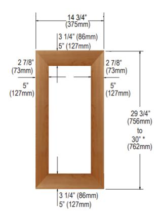
WHEN INSTALLING WITH THE HINGE SIDENEXT TO A WALL -
