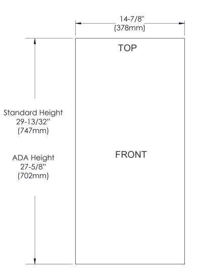
PANEL HEIGHTS ARE MINIMUMS, PANEL MAY BE TALLER. PANEL MUST NOT INTERFERE WITH TOEKICK VENTS. AFTER INSTALLATION UNDERCOUNTER DOOR MUST BE ABLE TO OPEN 90°
