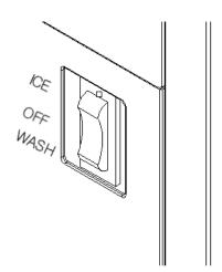
Turn the appliance to ICE, this will start the ice making process.
