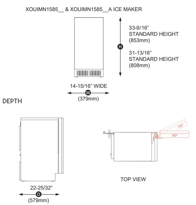
THE OVERALL DEPTH SHOWN (22-25/32") INCLUDES THE DOOR WITH 3/4" PANEL. THE DEPTH OF THE ICE MAKER CABINET ONLY IS 20-13/32"
