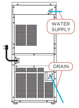
IMPORTANT: The keep drains as short and straight as possible for optimal performance.
