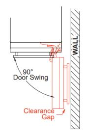
When installing with The hinge side next to a wall - Leave adequate space for your door handle.
