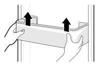
**2** To assemble the bin, slide it in above the desired support and push down until it snaps into place.
