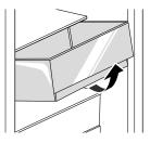
**2** To reassemble, slightly tilt up the front, insert the crisper into the frame and push it back into place.
