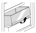
To assemble drawers, slightly tilt up the front, insert into the frame and push back into place.
