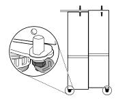
Open the door and use the wrench to loosen the keeper nut by turning it to the left.
