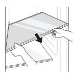
2 Pinch the sides to open the water filter cover.
