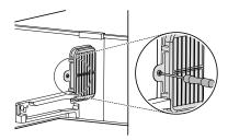
Press on the hooks at the air filter and then take it out.
