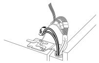
Hold the water supply connection and gently push in the collet **5** to connect the water supply lines as shown. Insert the tube at least 5/8 inch (15 mm) into the connector. Insert the clip on the joint to fasten the tubes in place.
