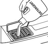
**IMPORTANT:** Do not use chlorine bleach or powdered detergent in the bulk dispenser. Powdered detergent must be added to the single-load dispenser.
