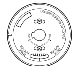
Back of OVEN TEMP knob (knob appearance may vary)
