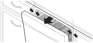
Open door and check that space between dishwasher cabinet opening and tub is equal on both sides. If spacing is not equal, loosen bracket screws and shift tub. Tighten bracket screws.
