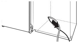
**NOTE:** Pull slack out of utilities at the same time the dishwasher is pushed into the cabinet opening to avoid any kinks.
