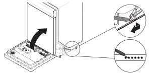
If the door closes too quickly, decrease the spring tension by moving the spring end toward the front of the dishwasher. **NOTE:** Springs should be in the same notches on left and right sides.
