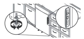
Check that leveling legs are firmly against the floor. Close and latch the door and place level against the front panel. Check that dishwasher is centered from front to back in the opening. If needed, adjust leveling leg until dishwasher is plumb. Repeat for other side of dishwasher.
