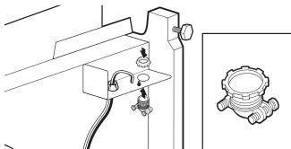
Install the metallic strain relief provided in this kit (Straight: Whirlpool Part Number 4317824, 90°: Whirlpool Part Number W10278923RP). Make sure screw heads are facing to the left when tightening conduit nut. Strain relief is provided with the power cord kit.
