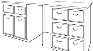
Measure height of cabinet opening from underside of countertop to floor where dishwasher will be installed. Be sure to measure the lowest point on the underside of the countertop and the highest point on the floor.
