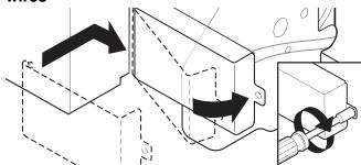
Place wires inside terminal box. Insert tabs on left side of cover. Make sure wires are tucked inside box. Close cover ensuring wires are not pinched. Use 1/4" nut driver or Torx<sup>®</sup> T20<sup>®</sup> screwdriver and previously removed screw to secure cover.
