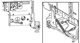
Select products include a factory installed power cord. For these products, no wiring during install is required. A ground wire to chassis connection is made inside the existing terminal box, and the normal terminal box cover is not included.
