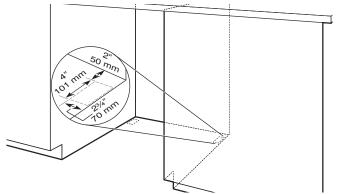
Built-up floors: If the kitchen floor is higher than the cabinet opening's floor—for example, the kitchen floor tile does not extend into the cabinet opening—add shims, as needed, in the area shown to bring the dishwasher up to 34" (864 mm) below the countertop.
