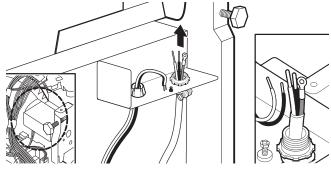
Route cord so that it does not touch dishwasher motor or lower part of dishwasher tub. Pull cord through strain relief in terminal box.
