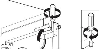
Place wires inside terminal box. Insert tabs on left side of cover. Make sure wires are tucked inside the box and not pinched by the cover. Use a 1/4" hex-head socket, nut driver, or Torx® T20® screwdriver, and the screw removed in step 22 to secure the terminal box cover.
