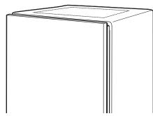
Cut insulation blanket along perforation for cabinet opening height of  $33^{1/2}$ " (851 mm). For other cabinet opening heights, do not cut the insulation blanket.
