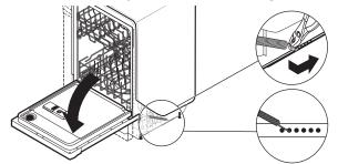
If the door falls open, increase the spring tension by moving the spring end toward the back of the dishwasher. **NOTE:** Springs should be in the same notches on left and right sides.
