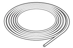
If using copper tubing, measure overall length of copper tubing required to reach the water supply, cut to length, and attach with compression fittings. 15. Slide nut and ferrule onto tubing (copper tubing only)
