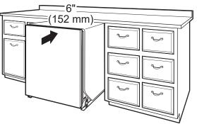
**NOTE:** Leave unit about 6" (152 mm) out from cabinet in order to install anchor brackets and adjust door tension if needed.
