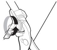
Be sure rubber washer is properly seated in fitting. Slide the 3/4" (19 mm) fitting of the 90° elbow up to the valve and hand-tighten to avoid cross-threading. Hand-tighten until the coupling is tight. Using pliers, check the tightness of the coupling. An additional 1/4 to 1/2 turn may be required to seal the rubber gasket. Route fill hose out the rear left side of unit.
