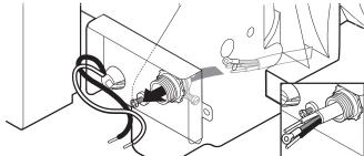
Route cable so that it does not touch dishwasher motor or lower part of dishwasher tub. Pull cable through UL-listed/ CSA-approved strain relief in terminal box. Strain relief is not supplied with the dishwasher. Owner must purchase a 7/8" (22 mm) screw-in type strain relief.
