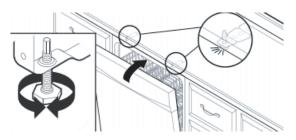
**IMPORTANT:** Check that top of door does not contact screws, brackets, or countertop. If it does, adjust leveling legs or use the side attachment option.
