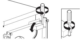
Using a 1/4" hex-head socket, nut driver, or Torx<sup>®</sup> T20<sup>®</sup> screwdriver, remove terminal box cover. Retain for later use.
