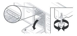
Place level against top-front opening of tub. Check that dishwasher is level from side to side. If dishwasher is not level, adjust front legs up or down until dishwasher is level.
