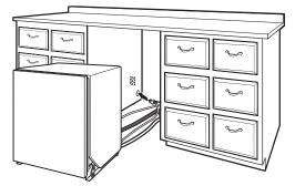
If using a power cord, make sure to route end through hole in cutout before sliding dishwasher into cabinet opening.
