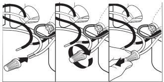
Select UL-listed/CSA-approved twist-on wire connectors of the proper size. Connect wires, black to black and white to white, using the twist-on wire connectors.
