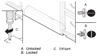
Using a flat-blade screwdriver, turn the fasteners 1/4 turn clockwise to lock into place. The fastener slot will be straight up and down when properly locked. Go to step 66.
