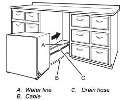
Route the utilities through the holes in the cabinet and pull the slack out at the same time as the dishwasher is pushed into the cabinet.
