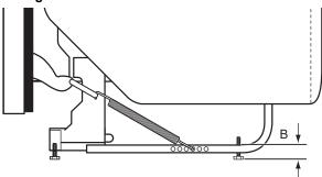
Adjust both front and back leveling legs to the same height. **NOTE:** If the minimum cabinet opening height is less than  $33^{7}/_{8}$ " (860 mm), the rear leveling legs and spacers can be removed for additional clearance. This will allow the dishwasher to fit into a  $33^{1}/_{2}$ " (851 mm) high cabinet opening, but the dishwasher will be more difficult to move. (Measurements are approximate. Rear and front leveling legs are preset at the factory for  $34^{1}/_{2}$ " [876 mm].)
