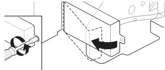
Using a 1/4" hex-head socket, nut driver, or Torx<sup>®</sup> T20<sup>®</sup> screwdriver, remove terminal box cover. Retain for later use.
