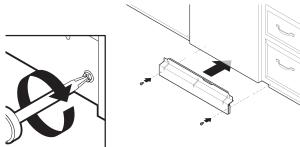
Place the panel against dishwasher legs. Using a Phillips screwdriver or 1/4" nut driver, reinstall the screws through the holes in the access panel.
