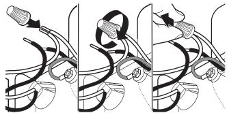
Select twist-on wire connectors of the proper size provided in this kit (Straight: Whirlpool Part Number 4317824, 90°: Whirlpool Part Number W10278923RP) . Connect wires, black to black and white to white, using the twist-on wire connectors.
