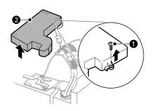
Disconnect all wire harnesses 3. Unscrew the ground wire 4. Remove the cover.
